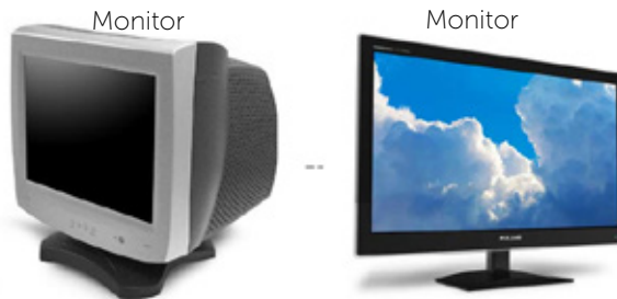
FIGURA 14 – COMPARATIVO MONITOR CRT X MONITOR FLAT-PANEL
